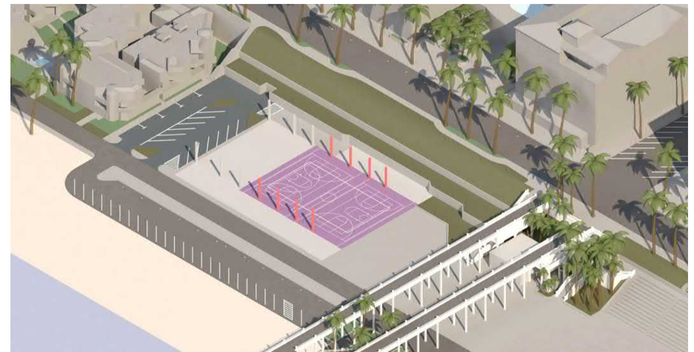
COURTS REBUILT AT SOUTH END OF BUILDING Shifting the new court space south on the property, allows some of the existing building structure on the north side to remain. The stage is demolished and this area is renovated for new program use. Assembly functions can be accommodated with retractable seating and a movable stage located at the court space when needed.
