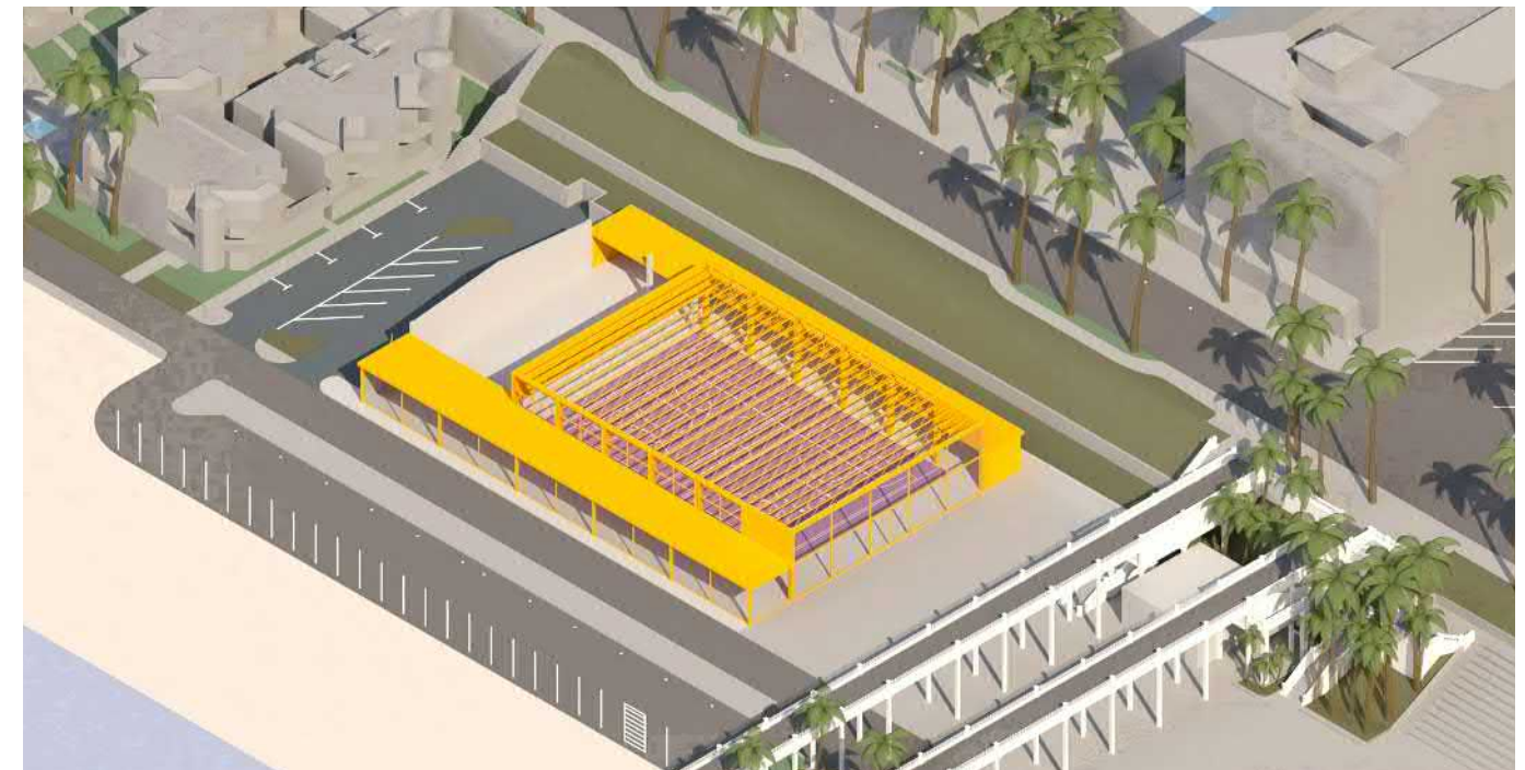
NEW STRUCTURE A new structural system, illustrated in dark yellow, with a wider span and taller columns is required to enclose the larger and higher court area. The taller structure exceeds maximum height prescribed by Proposition A. The single story flanking building areas must be restructured to meet current structural codes, with new steel members, foundations and other structure required to strengthen the lateral force-resisting system.
