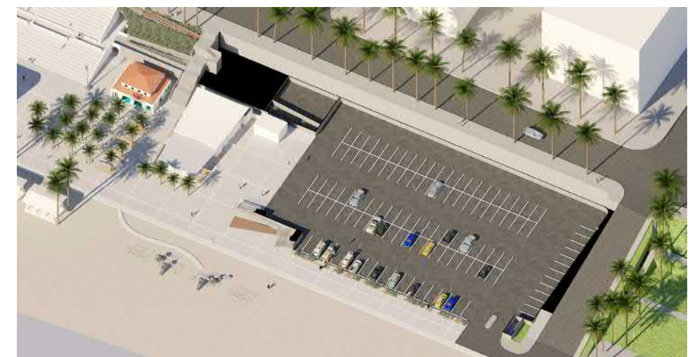
Strand-Level View: Parking remains at existing grade, below the park, and spaces are increased from 111 to approximately 128 spaces. The Strand vehicular right-of-way is maintained for the full length of the site as it exists.
