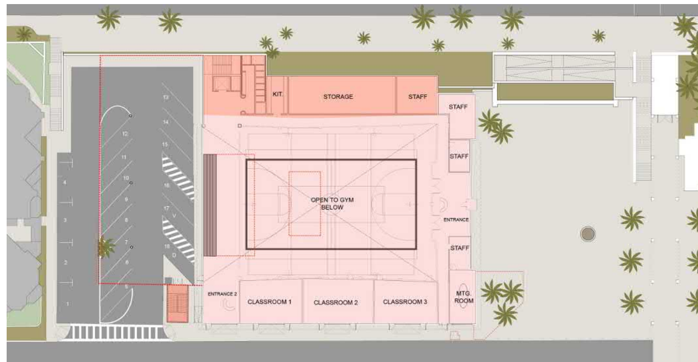
OPTION C RENOVATION/MAXIMUM ADDITION Ground floor plan illustrating first floor addition on the east side of the building. Included in the addition, are storage areas, restrooms, and stairs and elevator to a proposed new second floor addition located over the existing parking lot.
