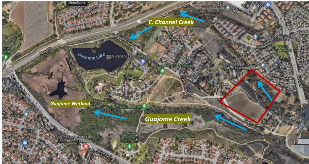
Figure 3. Drainage Patter around Property
