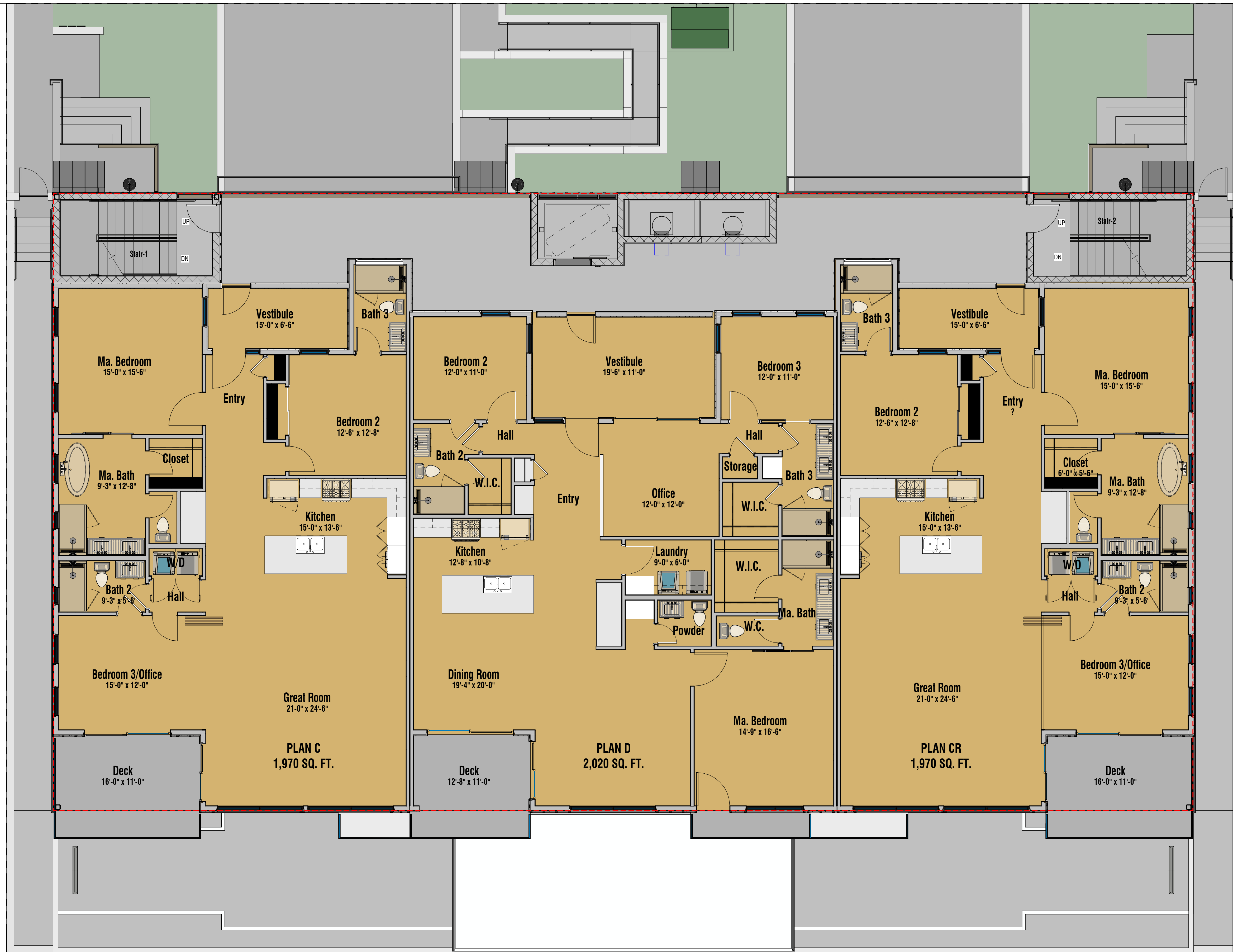
3RD LEVEL FLOOR PLAN 3/16" = 1'-0"
