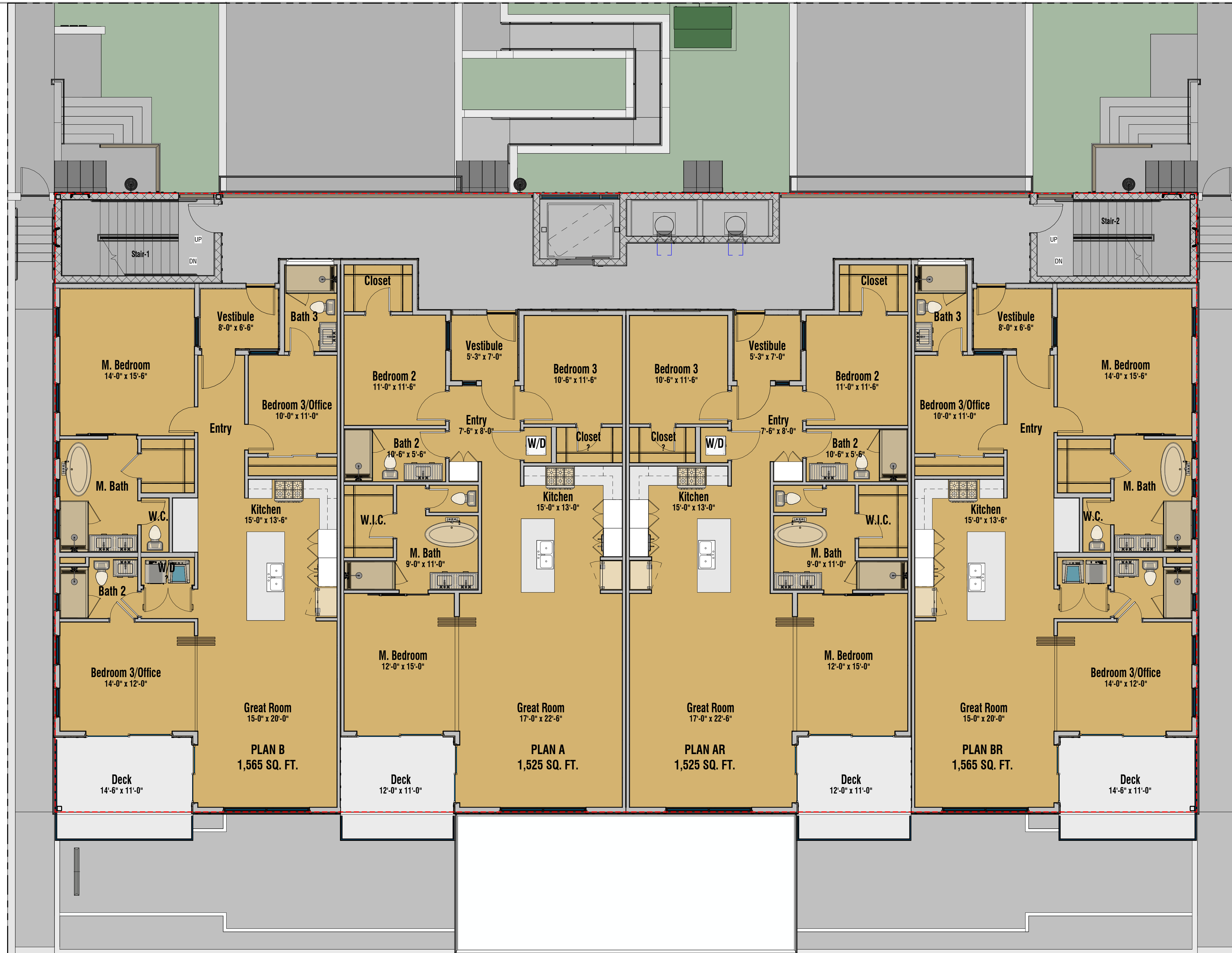
2ND LEVEL FLOOR PLAN 3/16" = 1'-0"
