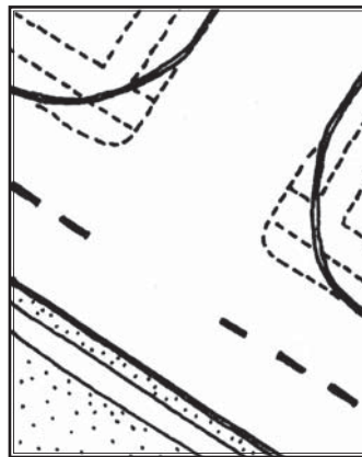
7S) Wide radius corners can promote high speed turning movements that can conflict with pedestrians. A high speed right turn can also take the driver's focus away from the crossing and its users and place the focus only on vehicles approaching from the left instead of pedestrians in the crosswalk. Photo credit: Michael Ronkin
