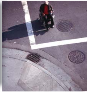
1A) Apex ramps (single ramp on corner), should be avoided on high volume streets with travel lanes at the curb. Photo credit: Dan Burden
