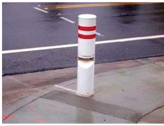
11S) A traffic signal or special pedestrian crossing can be controlled by sensors that note when a pedestrian approaches and / or leaves an intersection or a mid-block area. Photo credit: Michael Ronkin
