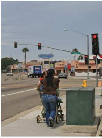
15S) Sidewalks placed against the curb, against a high speed and high volume street are not comfortable to walk on because of a fear (perceived or real) of being hit by a passing vehicle. Photo credit: Mike Singleton
