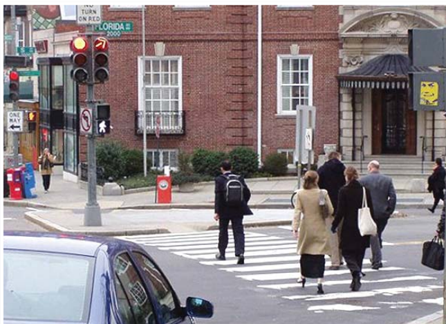
8S) Right turn on red restrictions with an advance lead for the pedestrian crossing phase can reduce right hand turning conflicts. Photo credit: Michael Ronkin
